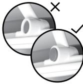
1. Place tub upside down and unfold both support legs outward until they snap into their locked positions.
