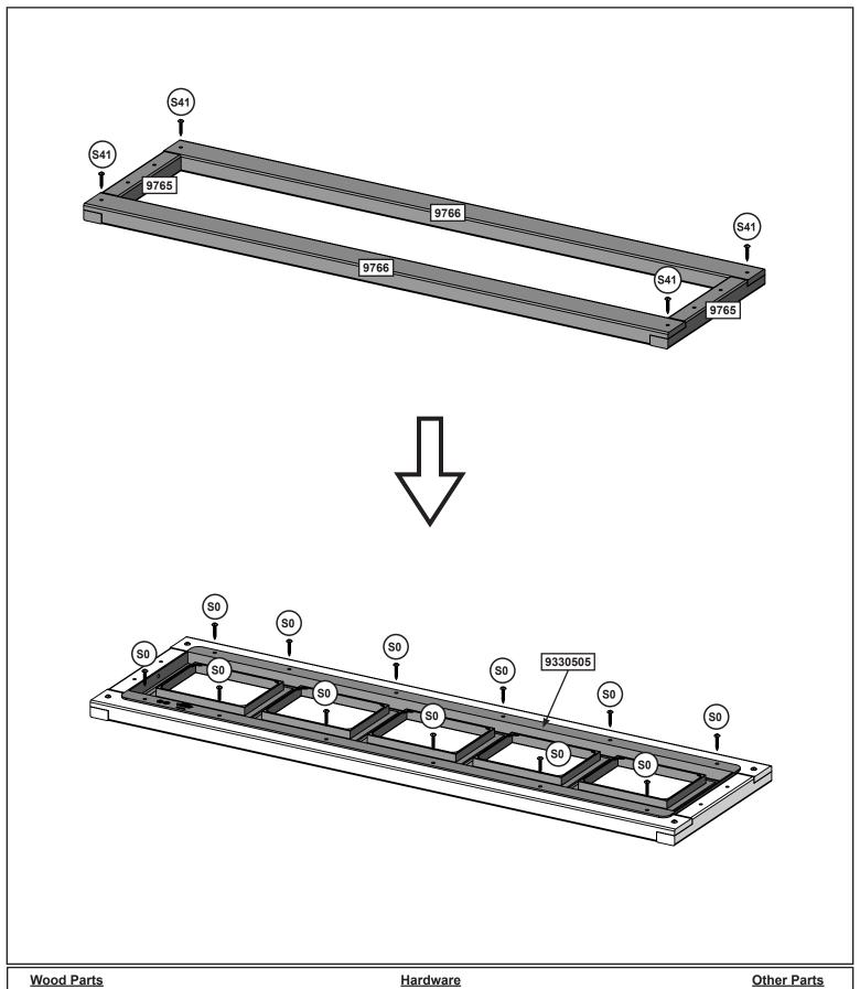
4 x 9765 25.4 x 30 x 279.4 mm (1 x 1-3/16 x 11") 4 x 9766 25.4 x 50.8 x 971.6 mm (1 x 2 x 38-1/4") 24 x so #8 x 22.2 mm (#8 x 7/8") 8 x s41) #8 x 22.2 mm (#8 x 7/8")
