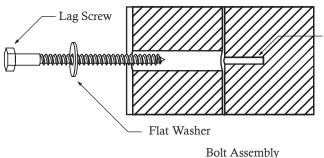
Before mounting Lag Screw, use factory drilled holes as guides to drill 1/8" pilot holes
