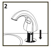
Feed the data cable (a) and the shank of the dispenser assembly (1) through the hole in the countertop. Point the spout of the dispenser into the sink bowl and press down firmly on the dispenser to securely attach it to the counter top.
