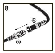
Connect the two halves of the data cable (6a) and (6b) by lining up the white stripes on each half and pushing the cable connectors together until the stripes touch.
