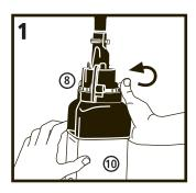
Grasp the empty refill bottle ① with one hand and use the other hand to push the green release latch on the motorassembly/bottle support ⑧ to the right (counterclockwise as seen from above).
