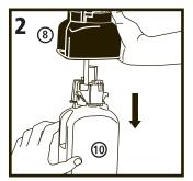
While still pushing the green release latch, pull downward on the refill bottle (1) and remove it from the motor assembly/bottle support (8).
