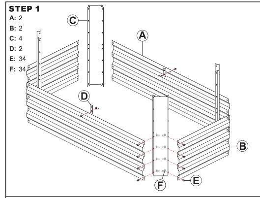
**IMPORTANT:** Ensure Long Panels (A) are installed in the correct direction, with the mounting holes toward the center and the rolled edge facing inward.
