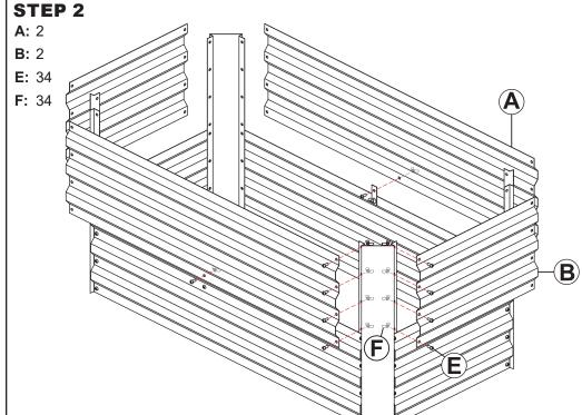
Align and loosely secure the remaining Long Panels (A) and Short Panels (B) using Bolts (E) and Wing Nuts (F).
