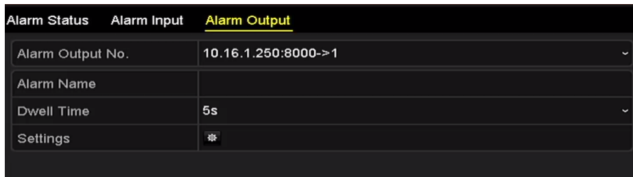
Figure 8-19 Alarm Output Settings Interface
