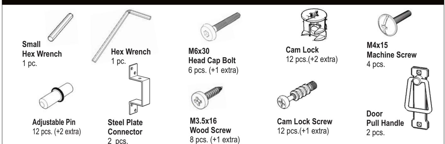
Tools required for assembly : Phillips screwdriver
