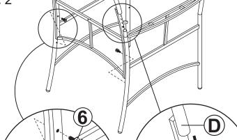
Do not fully tighten hardware until after Step 2 is complete.
