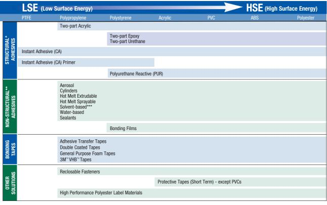
NOTE: The optimal curing guideline for plastics solutions ranges from 72 hours to 7 days. \* Structural strength adhesives reach a minimum of 1,000 psi overlap shear strength. \*\* Non-structural strength adhesives typically reach less than 1,000 psi overlap shear strength.
