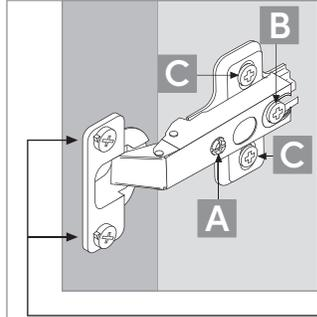
**Use screw A for horizontal adjustment, screw B for depth adjustment and screws C for vertical adjustment.**
