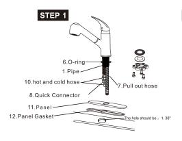
Position the faucet, deck plate and o-ring on the installation surface.
