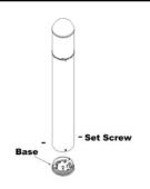
5 if NOT using NICOR provided anchor bolts, remove knockouts from base plate.
