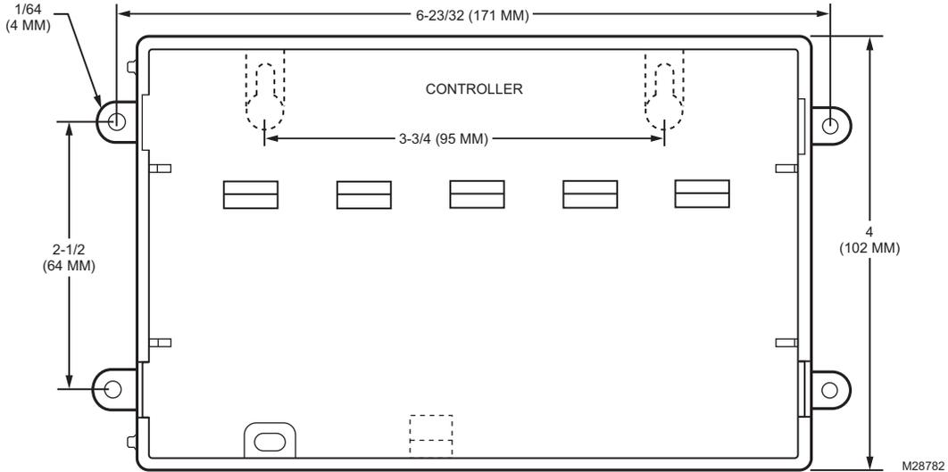
Fig. 2. Controller mounting tab dimensions in inches (mm).
