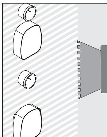
Install the tile or other finished wall material over the sealing gasket.
