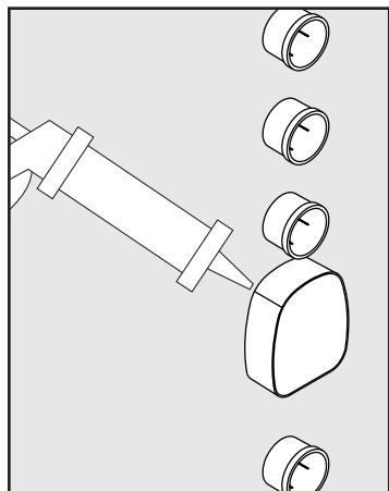
Install the sealing gasket(s).
