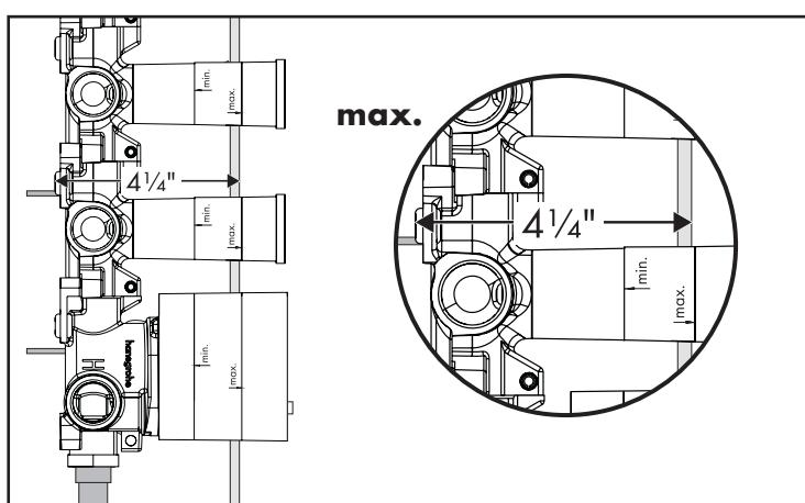
**! The outside surface of the finished wall must fall between the "min" and "max" markings on the plaster shields.**
