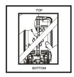
For proper dispenser tape adhesion: Press firmly all around backplate as shown in figure for 30 seconds.
