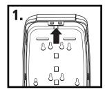
Open dispenser by pushing on cover latch until it releases.
