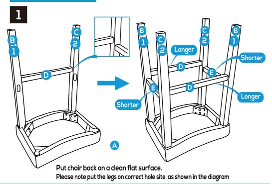
Align front legs in the seat pad as shown in the diagram.
