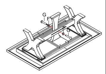
Step 5: Insert wood plugs (G) with plastic washers (F) into center pedestal through stretcher, tighten wood plugs by turning in clockwise direction.
