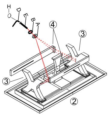
Step 3: Attach stretchers (4) to side pedestals (3), and use metal caps (H) to cover bolts (E).
