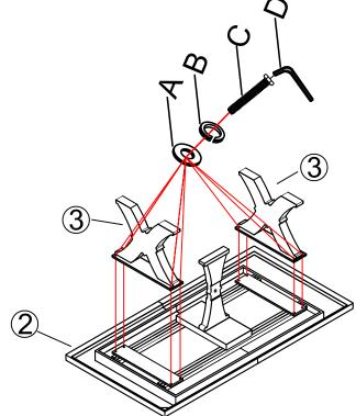
Step 2: Attach side pedestals (3) to table top (2).
