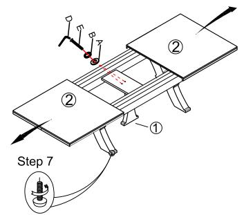
Step 6: Turn table upright and pull out table top, tighten center pedestal (1) by using flat washers (A), lock washers (B), bolts (E) and alllen wrench (D).
