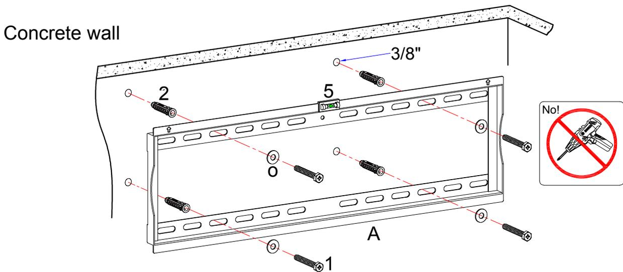
Figure 2 (keep the Wall plate level)
