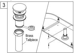
3. If you have access to the tub drain from below the floor, apply Teflon tape to the drain and thread the included tailpiece, measure the distance that it protrudes from the bottom of the tub and rough in your drain pipe accordingly.
