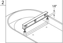
2. Adjust feet so that they protrude 1/8" below the level of the tub, you can accomplish this by placing a level or a straight piece of lumber across the width of the tub.
