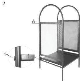
• Fasten remaining Side Panel (A) to the bottom bars by hand-tightening two M6x30mm Bolts (1).
