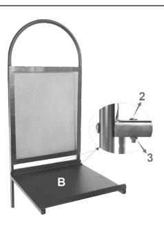
With the ledge facing upward, and flush with the side panel, secure Bottom Panel (B) to the bottom bars using four M5x25mm Bolts (2) and four M5 Nuts (3).
