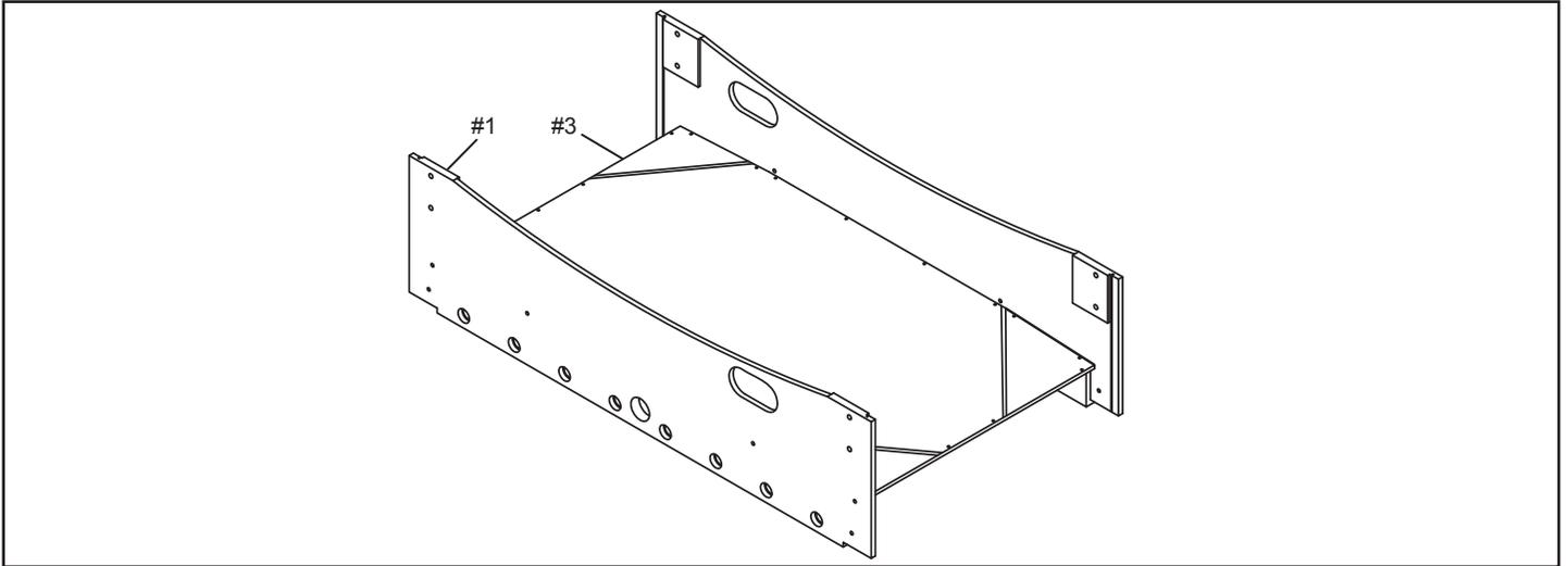
2. Attach one END PANEL #2 to each end of the table with 1/4" BOLT #10 and 1/4" FLAT WASHER #8.
