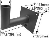
180° Wall Mount Bracket with 2-3/8″ O.D. Tenon OPL41WM1 MAX EPA: 0.5 Finish: Dark Bronze The 180° wall mount bracket with 2-3/8″ tenon attaches flood and area fixtures to almost any surface: wall, roof, or wood pole. Provides wiring access and a built-in 2-3/8″ O.D. tenon to mount a fixture with our adjustable slip-fitter. Suggested 3/8″ diameter bolts for mounting.
