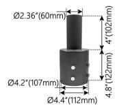
4" Round Pole Mount with 2-3/8" O.D. Tenon OPL41TNA MAX EPA: 0.3 Finish: Dark Bronze For use with round, non-tapered steel and aluminum poles. Furnished with four 3/8" hex head stainless-steel bolts. Vertical tenon measures 2-3/8" O.D.
