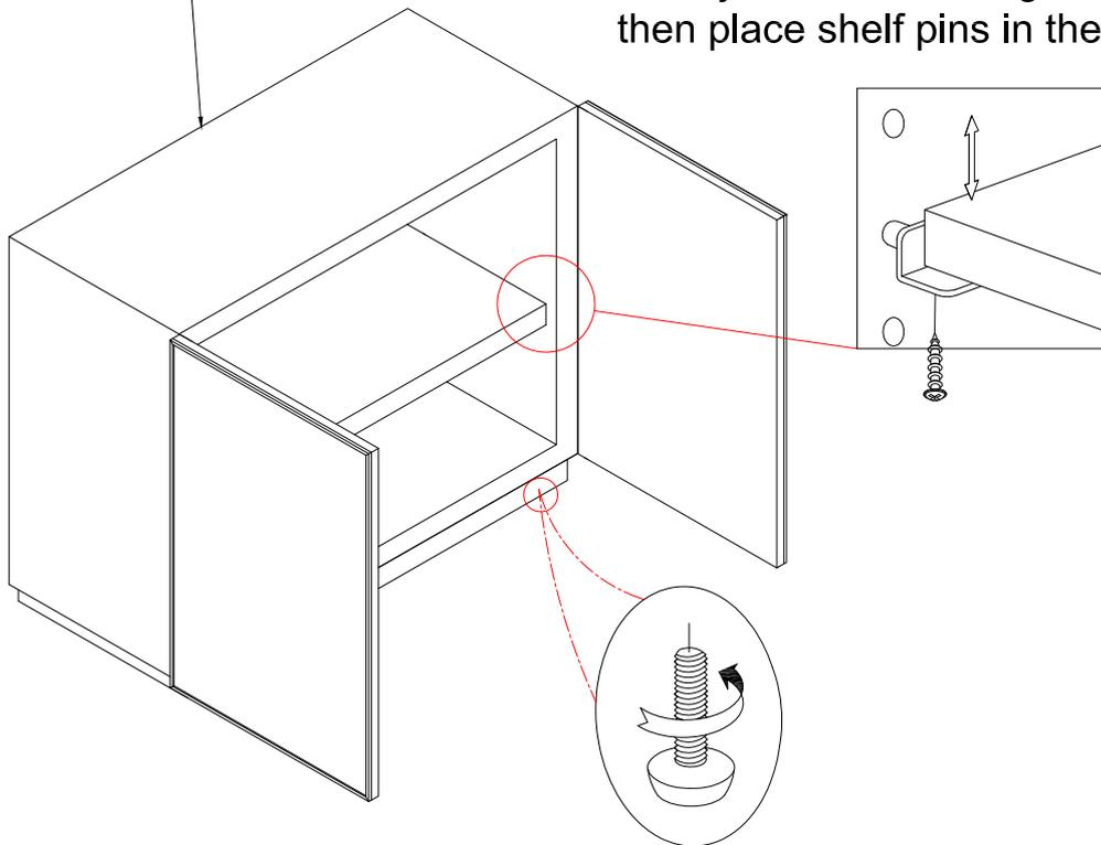
Adjust leveler if needed to level the case on uneven floor.
