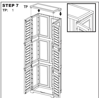
Ensuring the pivot pins on the top doors align with the front of Top Panel (TP), firmly press the top to secure it to the unit.
