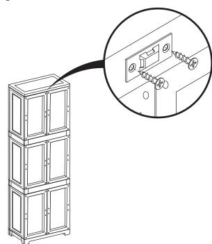
Secure one mounting tab to the back of the top panel using the short screws.
