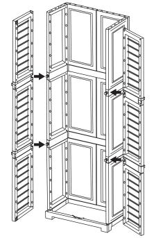
Align the pivot pin on the bottom door with designated hole on the bottom panel of the cabinet. Then, firmly press the back of each door handle onto the cabinet hinges.
