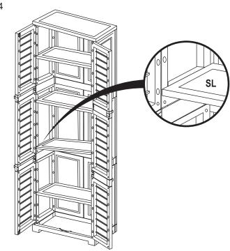
Install Shelves (SL) into the unit at a slight angle and align the shelf with one side of the unit. Then, gently press on the opposite side down until the shelf locks into place.
