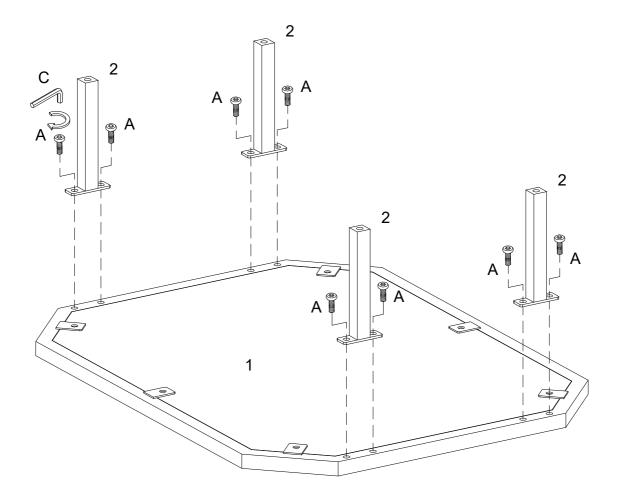
Using bolt (A) attach parts (2) to part (1) with Hex key (C) as per diagram. Note: Please do not fully tighten all bolts.
