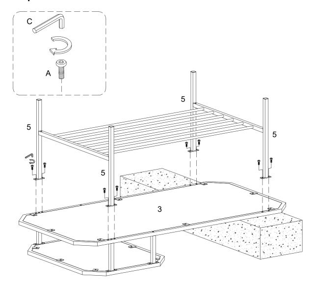
Using bolt (A) attach parts (5) to part (3) with Hex key (C) as per diagram. Note: please fully tighten all bolts .
