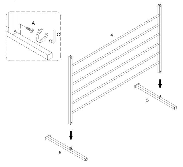
Attach part (4) to part (5) ,then using bolt (A) secure part (4) to part (5) with Hex key (C) as per diagram.
