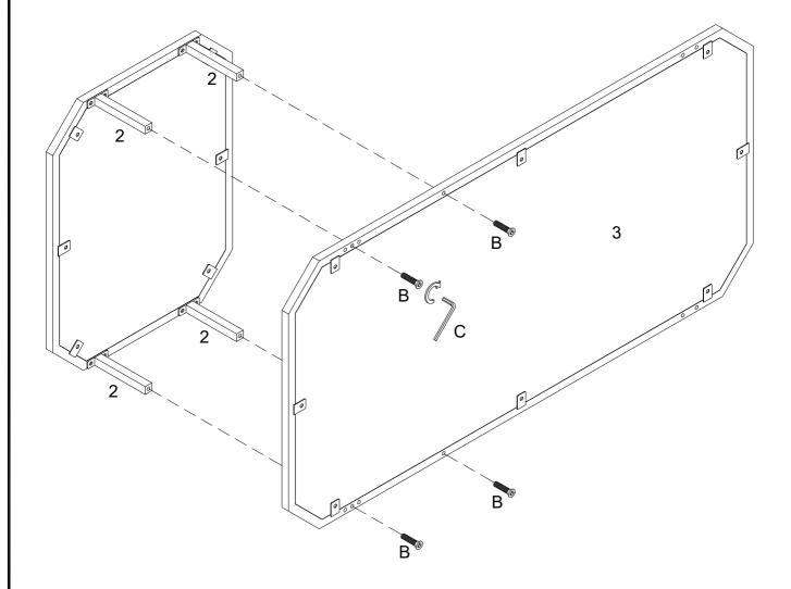
Using bolt (B) attach part (3) to part (2) with Hex key (C) as per diagram. Note: please fully tighten all bolts at this step .
