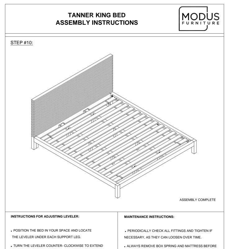
• ADJUST EACH LEVELER UNTIL EACH SUPPORT LEG IS APPLYING EQUAL, UPWARD PRESSURE ON THE BED SUPPORT SLAT.
