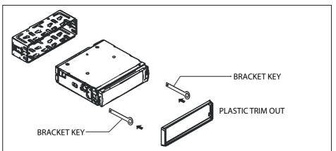
If you want to remove the chassis from the mounting sleeve, first remove the plastic trim out from both sides. Next, insert the two bracket keys into the left and right side of the chassis, as illustrated, to separate the chassis from the housing.
