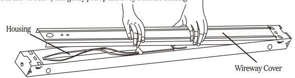
2)Locate the 2 sockets that are inside the housing, both have been prewired and are ready to be attached to the housing. Follow the five step-by-step illustrations shown below of how to attach the sockets, top plate and end plate to the fixture housing. Make sure that each piece is firmly in place before proceeding on.
