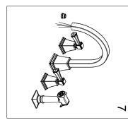
slightly to stop minor leaks. each. While water is running, check for water to run for at least one minute water supply and allow both hot and cold completed, remove aerator. Turn on 7.Important: After installation is leaks. Replace aerator. Tighten nuts
