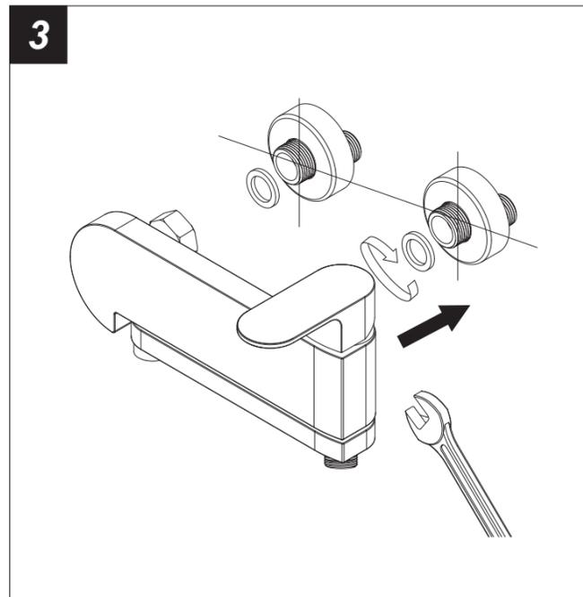
3. Install the faucet to the eccentric nuts as shown. Adjust the eccentric nuts if they do not match properly. Finally tighten by wrench.
