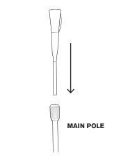
Fit the dual-wrapped tee top (A) onto the top of the main pole (B), with the tee cup pointing upward. The neck should slide to fit snugly in the main pole.
