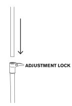
3. Slide the main pole into the base pole (D).
