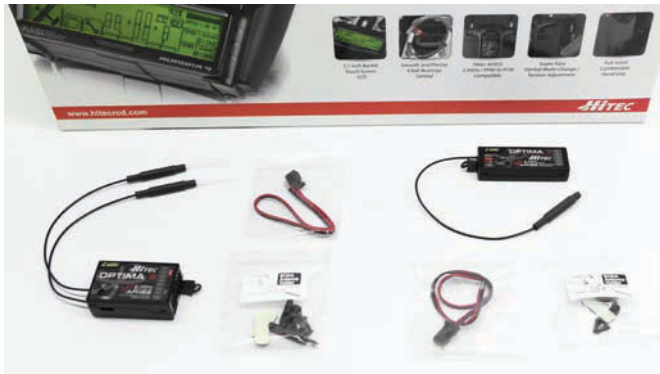
You have a choice of the dual-BODA Optima 9 and the single-BODA Optima 7; each receiver comes with an SPC power lead and BODA mounting kit
