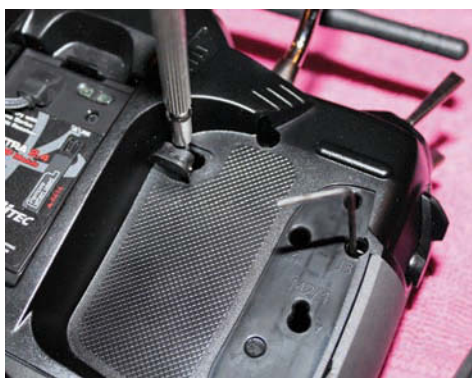
After removing the rubber grips, stick mode, tension and friction adjustments can be made without opening the transmitter case
