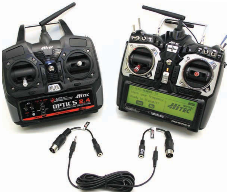
The Aurora 9 can be connected to 6-cell Optic transmitters using a simple 3.5 mm audio-plug lead (available separately); Hitec transmitters using 8-cells and DIN connectors will require the adapters available in the full-package cable set seen here
