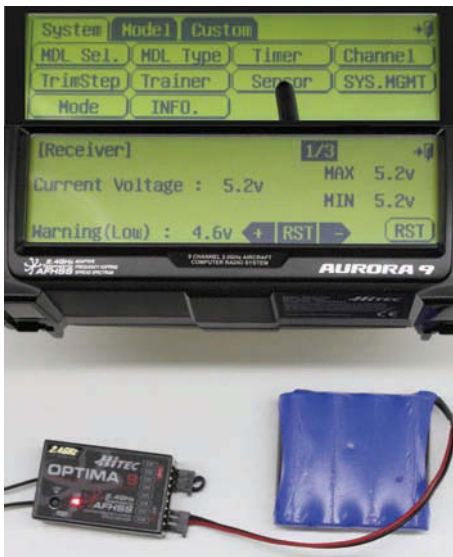
An example of the basic receiver voltage monitoring – available from the system tab's sensor function; more information is available if a sensor station with suitable telemetry sensors is connected
