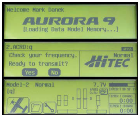
As the transmitter starts up it shows an initial screen then (optionally) asks if you wish to transmit (you might not want to while programming) before displaying the main status screen
