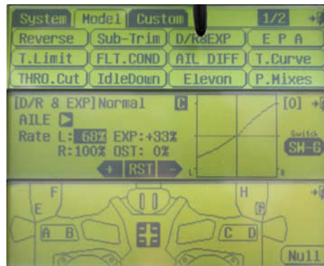
From the model tab the DR&EXP function calls up a graph and allows flexible setting of rates and expo; a further screen allows the choice of a switch to activate the function; using a 3-position switch allows a choice of multiple settings
