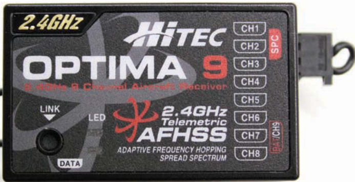
The compact Optima 9 has all the connections at one end and the data connection on the side
