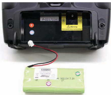
The standard 6-cell 1300 mAh NiMH can provide over 8.5 hours of operation if the LCD backlight is not left on
