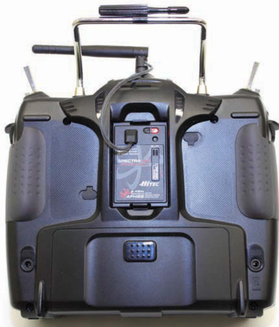
Rear view showing battery compartment flanked by charging socket and trainer/data port; a Spectra 2.4 module with external aerial lead is fitted to the Aurora 9; note the contoured rubber grips that provide a very comfortable grip, and a useful screwdriver/stylus is clipped to the carry handle
