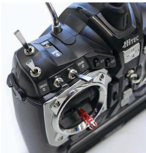
LHS auxiliary controls: four switches, a rotary/slider and two nudge buttons (LT, CT)
