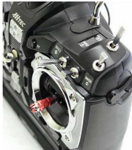
RHS auxiliary controls: four switches, a rotary/slider and one nudge button (RT)
