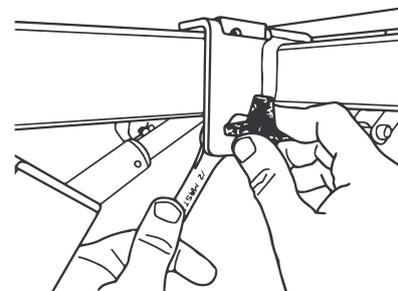
3. Tighten the cap screw with a half inch wrench while holding the knob with your other hand. Repeat for the other side.
