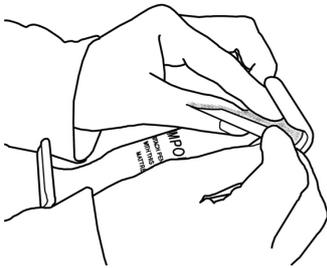
2. Position the hook and loop strip inside the cupped part of the pendant holster.
