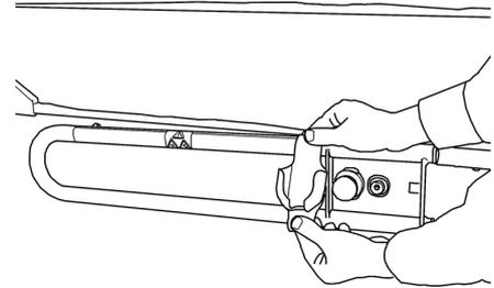
4. Place the pendant holster anywhere along the Assist Bar, between the two bars.
