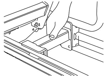
2. Position the Assist Bar bracket over the mounting tab on the frame.
