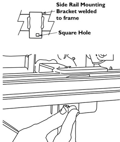
1. Insert the 5/16-18 x 3/4 Carriage Screw through the back of the frame-tab mounting hole.
