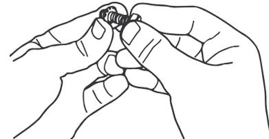
1. Insert the 5/16-18 x 1 cap screw through the 5/16 serrated washer.
