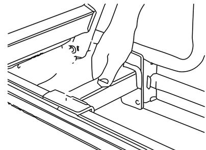
3. Lower the bracket to engage the mounting tab in the bracket slot.
