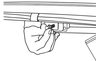
2. Place cap screw with washer through the back of the lower round hole in the side bar mounting bracket.
