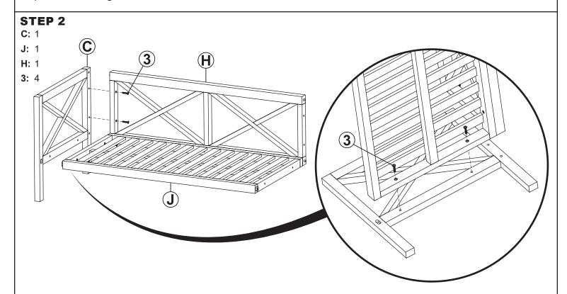
Loosely fasten one Lounger Backrest (H) to Right Panel (C) by hand-tightening two JCBC M6x35mm Bolts (3). Loosely fasten one Lounger Seat (J) to the right panel by hand-tightening two JCBC M6x35mm Bolts (3).
