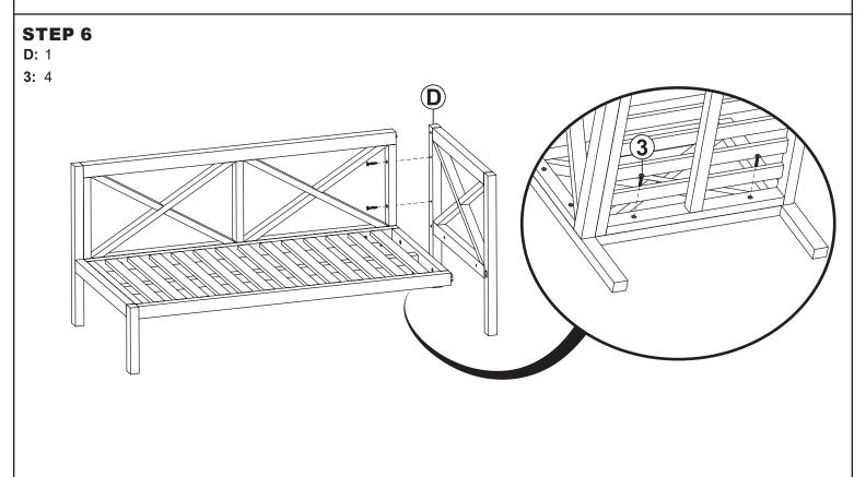
Loosely fasten the backrest and seat to Left Panel (D) by hand-tightening four JCBC M6x35mm Bolts (3).
