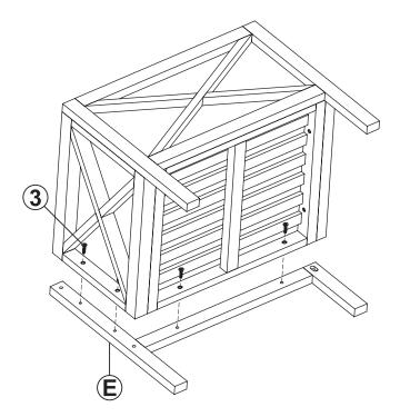
Securely fasten Left Leg (E) to the corner backrest and seat using four JCBC M6x35mm Bolts (3).
