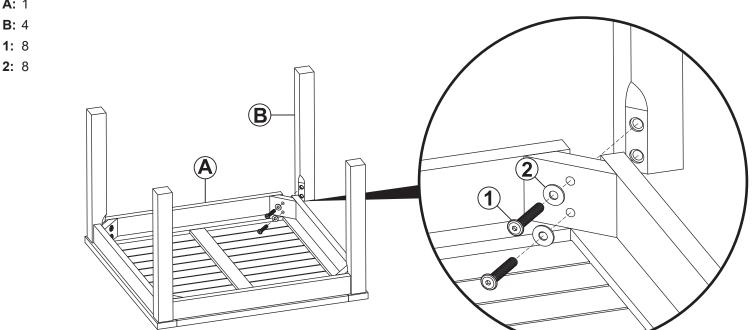
Securely fasten Table Leg (B) to Table Top (A) using two JCBC M8x45mm Bolts (1) and Washers (2). Repeat until all legs have been installed.
