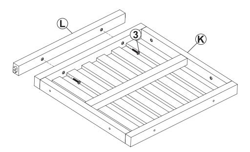
Secure Support Bar (L) parallel to the center crossbar of Corner Seat (K) using two JCBC M6x35mm Bolts (3).
