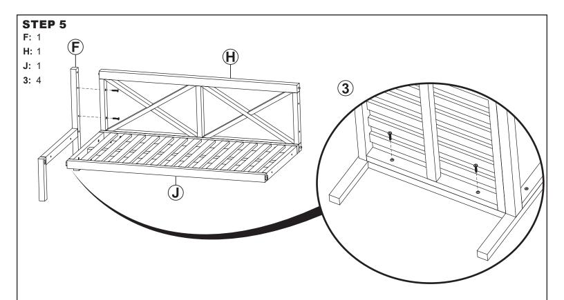
Loosely fasten one Lounger Backrest (H) to Right Leg (F) by hand-tightening two JCBC M6x35mm Bolts (3). Loosely fasten one Lounger Seat (J) to the right leg by hand-tightening two JCBC M6x35mm Bolts (3).
