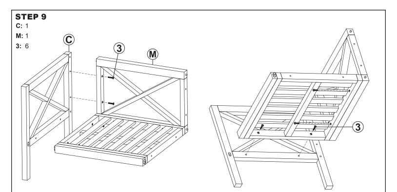
Loosely fasten Corner Backrest (M) to Right Panel (C) by hand-tightening two JCBC M6x35mm Bolts (3). Loosely fasten Corner Seat (K) to the right panel by hand-tightening two JCBC M6x35mm Bolts (3). Fasten the back of the corner seat to the backrest using two JCBC M6x35mm Bolts (3). Finish tightening all bolts.
