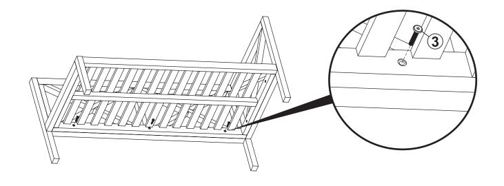
Secure the underside of the lounger seat to the backrest using three JCBC M6x35mm Bolts (3). Finish tightening all bolts.
