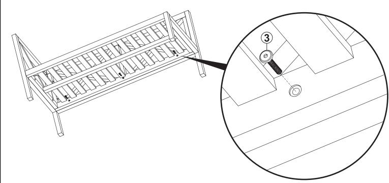
Secure the underside of the lounger seat to the backrest using three JCBC M6x35mm Bolts (3). Finish tightening all bolts.
