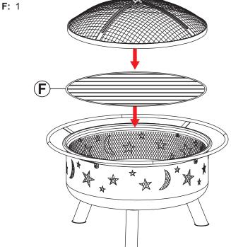
Place Cooking Grate (F) into the fire bowl and place the spark screen on the fire bowl.
