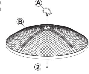
Secure Handle (A) to Screen (B) using one Flange Nut (2).
