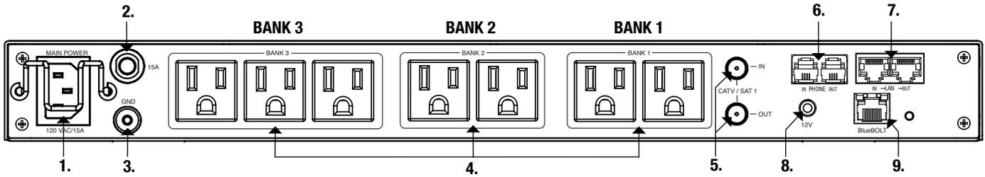
**1. AC Inlet:** 120 VAC, 15A, IEC 320-C13 do not remove steel retention clip.
