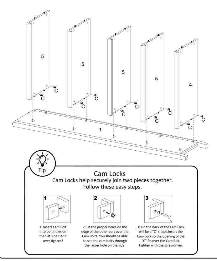
Attach Right Panel (2) to Shelf Panels (5) and (4). Secure with Cam Locks (C) and tighten with a screwdriver.
