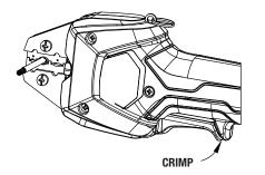
5. The crimp cycle will automatically stop when complete. Release the trigger upon crimp completion and the jaws will automatically retract.
