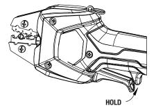
3. Insert the stripped wire into the connector.
