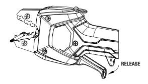
Note: The jaws may be manually released by pushing the trigger outward. This may be necessary if, for example, an incorrectly-sized connector has been inserted into the die opening.
