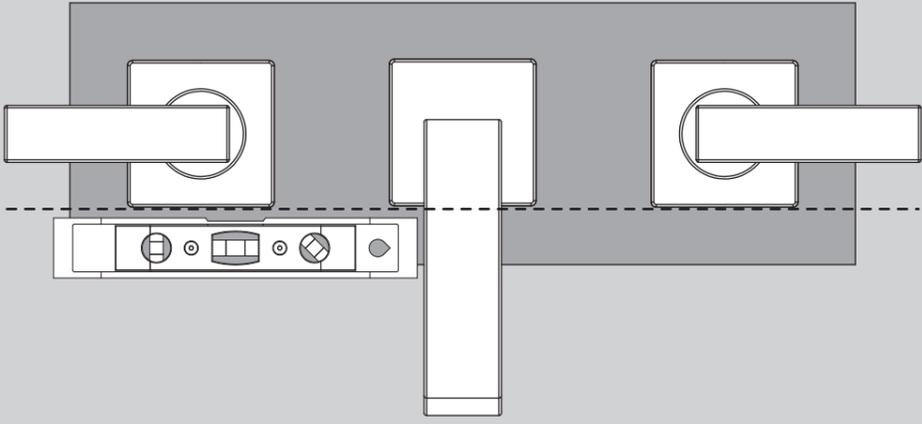
**7** While maintaining the proper alignment, Wrench Tighten Spout Mounting Nut (1). Then snug Endbody Mounting Nuts (2). Final tightening of Endbody mounting is accomplished by Tightening the Mounting Screws (3) while using a Phillips Screwdriver. Wrench tighten Spout Inlet Hose (4).
