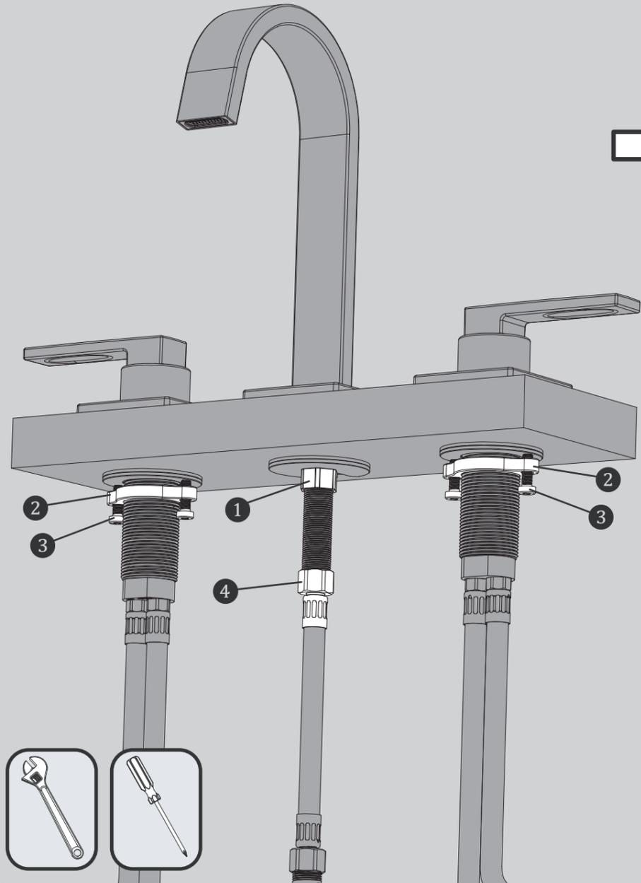
**8** From below, install the Endbody Outlet Hoses (1) (shorter hose) to the Inlet Tee of the Spout (2). Wrench Tighten. Wrench tighten Spout Inlet Hose (3) to Inlet Tee (2)
