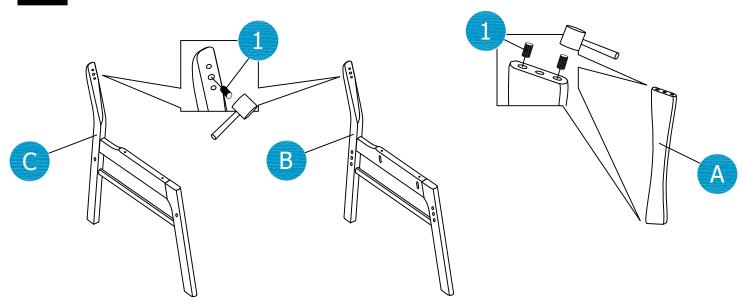
Assemble Part A front & back rail to Part B left chair side with 2pcs of part 2 screw,2pcs of part 3 spring washer and 2pcs of part 4 flat washer. Do not tighten screws too much at this stage.
