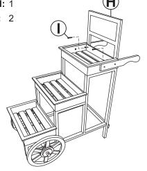
Loosely secure Top Tray (C) to the side panels using four M6x25mm Bolts (I).
