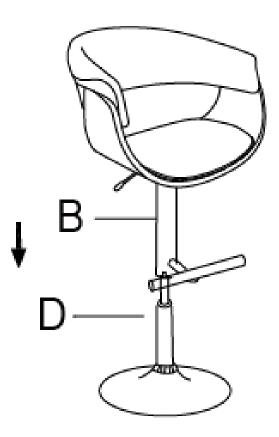
Place the assembled seat on Gas Lift (D). Please note the hole of the Footrest (B) should aim to the top of Gas Lift (D).
