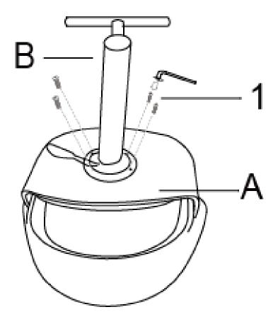
Attach Footrest (B) to Seat (A) using Allen Key Screws (1). Use Allen Key (2) to fully tighten.
