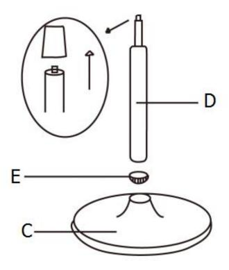
Remove the plastic cap from Gas Lift (D). Insert Gas Lift (D) and Plastic Ring (E) into the middle of the Base (C).
