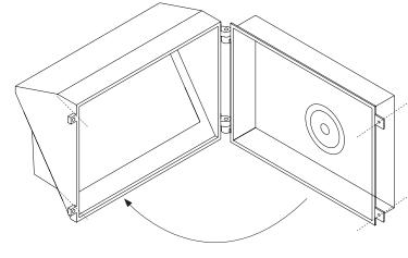
6 Open fixture and drill out the 0.28" holes for mounting to either (a) surface wall mount or (b) to a 4/O J-Box mount.
