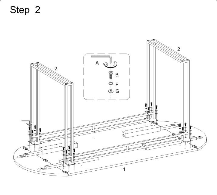
Using Bolt (B) attach lock washer (F) and flat washer (G) into part (2) to part (1) with Hex key (A) as per diagram.
