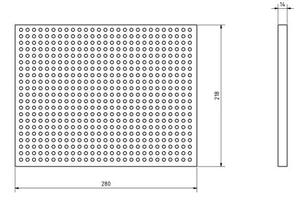
Filament Fine filter Filter surface: 0.061 m<sup>2</sup>
