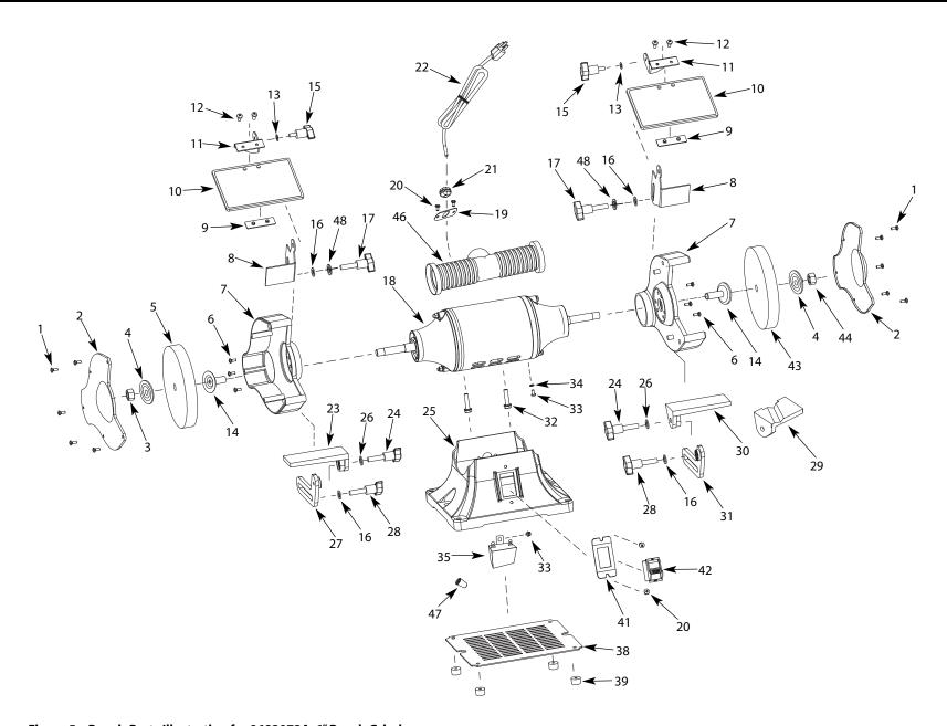
Figure 5 – Repair Parts Illustration for 9682072A, 6" Bench Grinder
