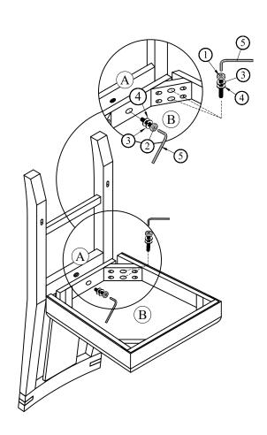
DO NOT TIGHTEN BOLTS COMPLETELY
