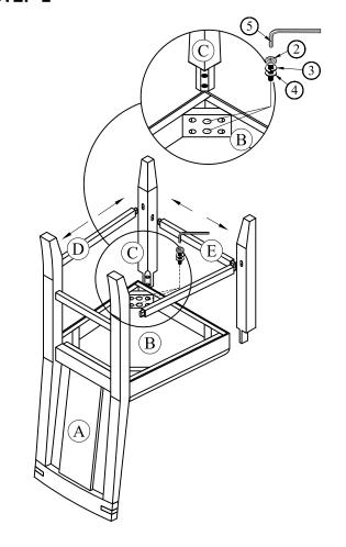
DO NOT TIGHTEN BOLTS COMPLETELY
