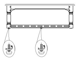
Step 4: Adjust leveler if needed to level table on uneven floor.
