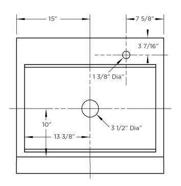
SINK TOP VIEW Showing Drain & Water Locations
