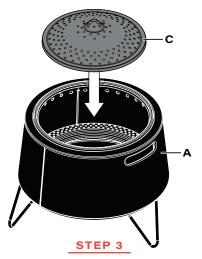
Replace the dome insert (C) into the Fire Pit.
