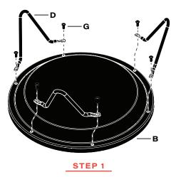
Secure each leg (D) to the ash pan (B) with 2 screws (G) using the supplied Hex Key.
