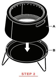
Place the fire pit (A) onto the lower assembly.
