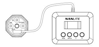
The fixture can be controlled by the wire controller in CCT mode, HSI mode, EFFECT mode, PIXEL FX mode, CHANNEL setting, LANGUAGE, DMX mode, DMX PIXEL, WIRELESS PROTOCOL, BLUETOOTH RESET, FIRMWARE UPDATE and VERSION checking (please refer to wire controller user manual for detailed instructions). (Note: Wire controller is sold separately.)
