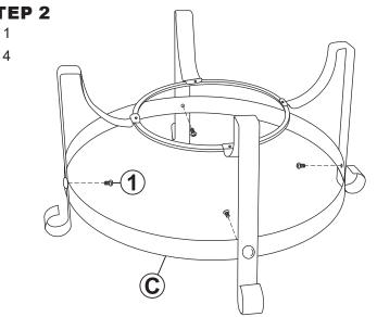
Align Large Ring (C) to the legs by hand-tightening three M6x8mm Bolts (1)
